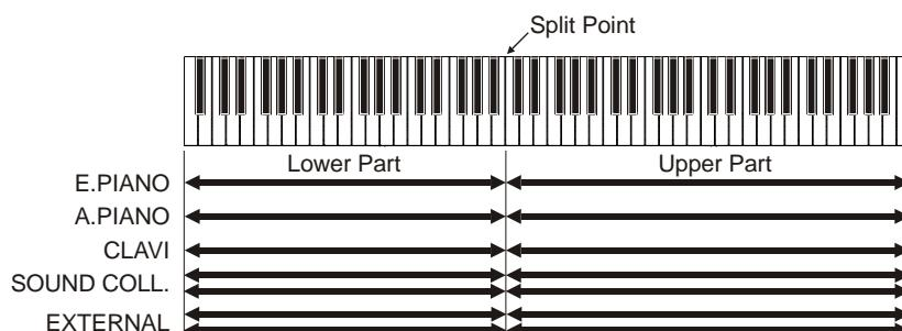
To assign a module to one of the parts, use the data entry dial or the [<>] and [<<] buttons to place the cursor on the line of the desired module, then press the dial.
