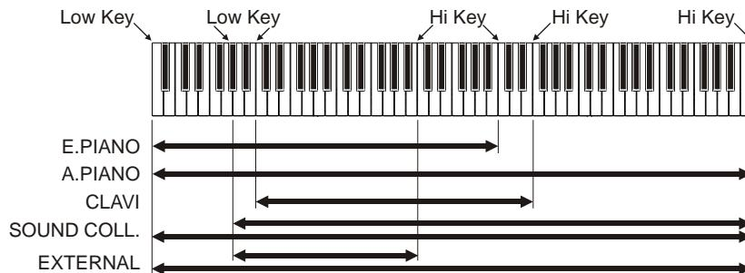
To select the *Lower Key* hold down the [<>] button and push a key. Hold down [<>] and press a key to select the *Upper Key*.
