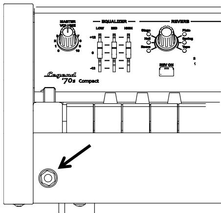
On the left side of the instrument, under the keyboard, you will find a 1/4" jack connector to plug in your headphones.
