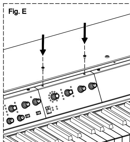
7. Fasten the bar to the top of the instrument and to the front panel by using the screws described at point 2.
