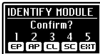
here you will find the module icons for a quick check of the modules positions. If the positioning of each module is correct, press the data entry dial to confirm. The message “Allocation Completed!” will appear on screen. Press [EXIT] instead to cancel and return to the *UTILITY* page.
