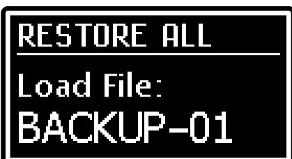
2. Turn the dial to select a backup file among those available on the USB drive and press the dial to load the file. The system will ask for a confirmation with the following message: “*Reset all data in internal mem. Are you sure?*”. If you accept, all the data on the instrument will be irreparably lost. Press the data entry dial to confirm or [EXIT] to abort.
