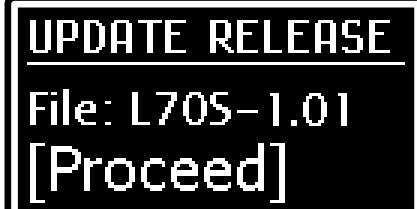
3. Make sure that this is the correct file, then press the data entry dial to start the update or press [EXIT] to abort the operation. Once the update has started, the system checks the file integrity and shows the message: "*Checking update...*". Then it loads the file, while showing the message: "*Updating...*" and the progress percentage. When the operation is over the message "*Update successful [Turn on/off]*".
