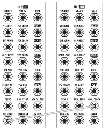
To Sync multiple DFAM units together, simply patch from the **TRIGGER** output on the Patchbay of the Primary unit, into the **ADV / CLOCK** input on the Secondary unit.
