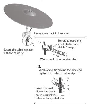
\* Take care to ensure that the cables do not touch the V-Cymbal pads and/ or the stand. A cable touching a V-Cymbal pad or a stand may cause double sounding or other incorrect operation.
